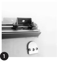
Remove end cap and put Adjustable bracket in place, using 1.5mm (0.06") hex key tighten adjustable bracket in plane (min. 2 per metre/40"). Reinstall end cap.
